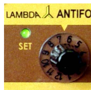
Figure 4: Control panel of the ANTIFO-controller.
