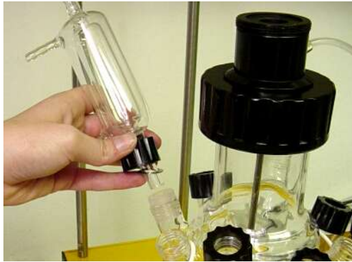
Fig. 12 Fixing of the glass air outflow cooler
