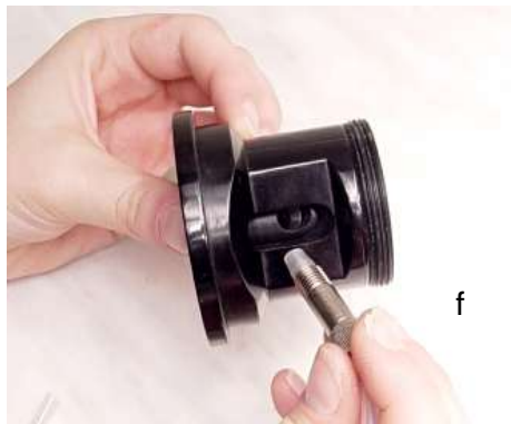
Fig. 5 The tubing is screwed into the cock head
