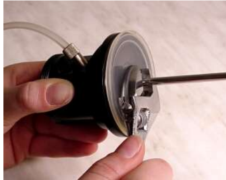
Fig. 7 Screwing the axis on the mobile part with membrane on the lower side of the cock head
