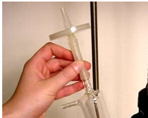
Fig. 13 The vent-filter is placed on the cooler
