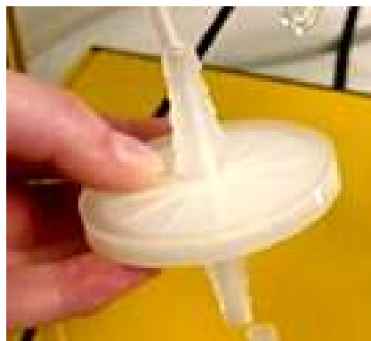
Fig. 6 The tubing is fixed to the corresponding filter.
