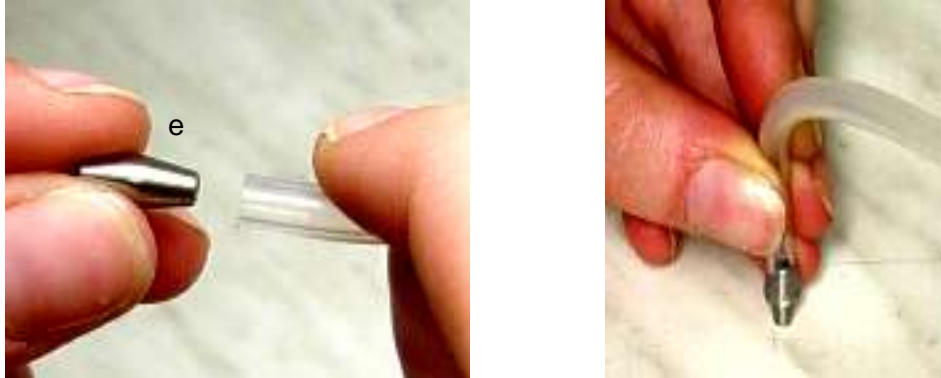
Fig. 4 A double-conical insert is placed into the tubing end
