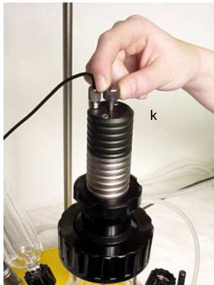
Fig. 16 Screwing of electromagnet
