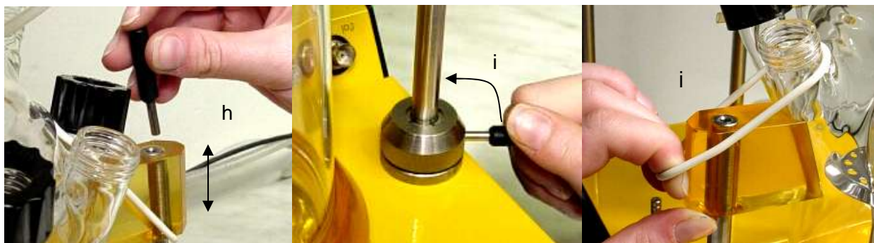
Fig. 11 Fixing the fermenter vessel onto the housing
